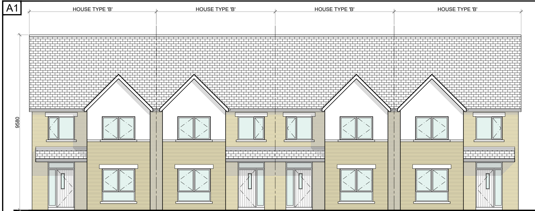
FRONT ELEVATION @ 1:100 TERRACE BLOCK TYPE 4
